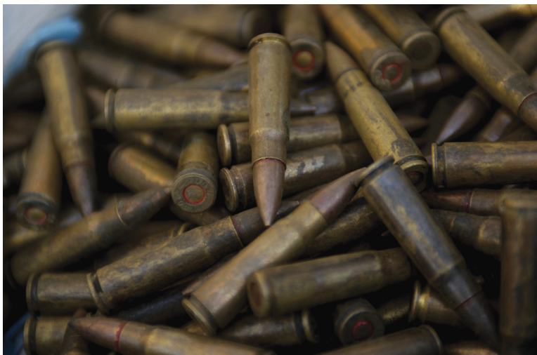
Figure 3.10 Ammunition under investigation in Baghdad, Iraq, in 2006. Closer inspection of the casing head stamp reveals ППZY for Prvi Partizan; the year 2002 is also marked. Other identifying characteristics to look at include the brass casing and the distinctively red primer sealant, a color unique to Prvi Partizan. (U.S. Air Force image; photograph by Technical Sgt. Adrian Cadiz.)
